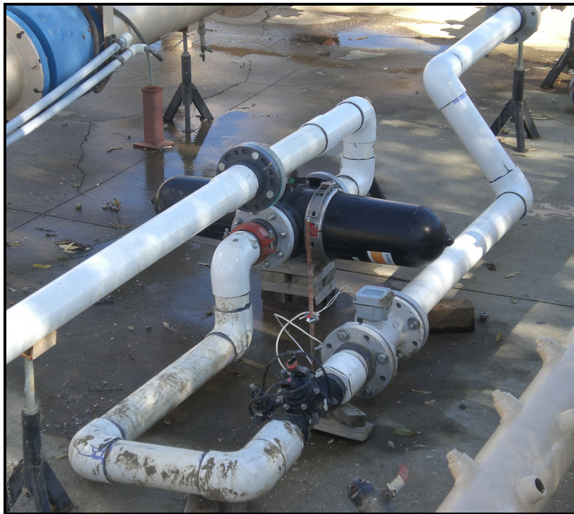
Figure 4. Test configuration for 4-inch magnetic meter
