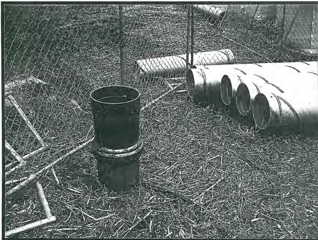
Mechanical Coupling - carbon to stainless steel
